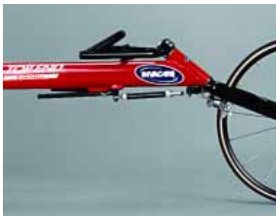
Oversized rake for maximum speed and aerodynamic steering for optimum control.
