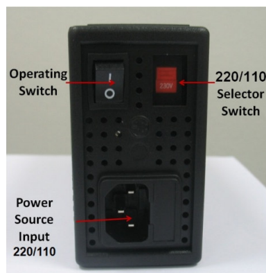
Figure 17 – Back panel of battery charger
