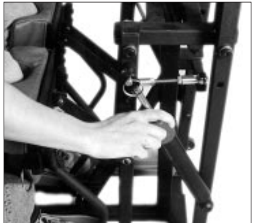
Adjust the level of the resistance cylinders while in the seated position. Start with #1 and work up.
