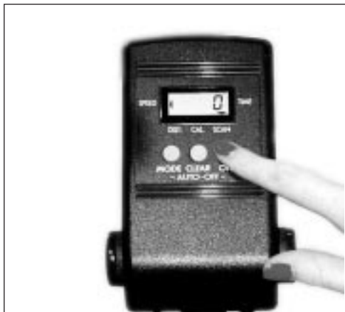
Simply push the “on” button, then continue pressing the mode button to reach desired operation.
